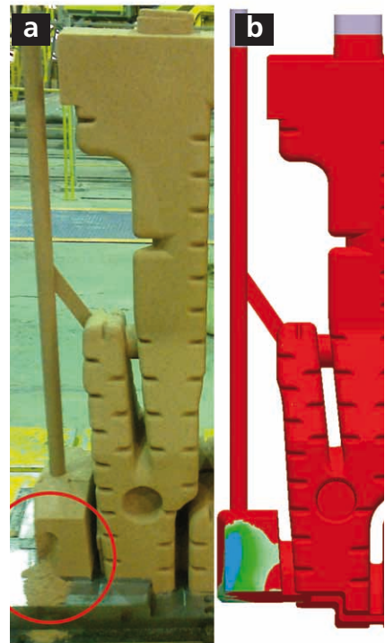
Figure 12: Shooting and gassing result with new process parameters: a) PUR cold-box core; b) predicted local concentration of absorbed hardening gas (red fully hardened, green critical, blue not hardened). The affected, unhardened area exactly corresponds to the predicted zone, with low amine concentration in the simulation result (blue)
