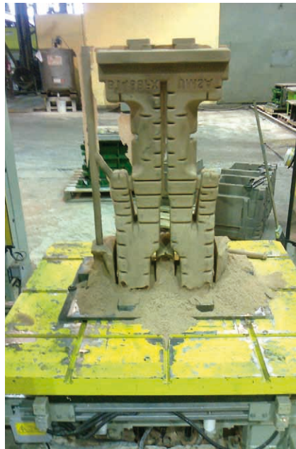
Figure 10: The first core-shooting experiment for a PUR cold-box core (length 920 mm, shooting volume 68 kg). The lower area of the core completely collapsed as a result of insufficient strength [10]
