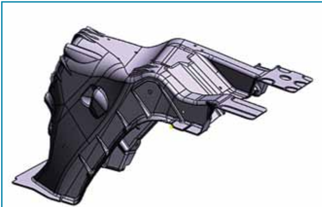
Figure 3: Front wheel shock tower of a passenger car. Initial problems with distortion being out of tolerance after casting and heat treatment were analyzed virtually.
