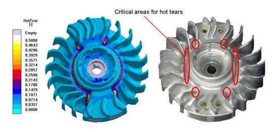
Figure 8: Prediction of areas with a tendency to develop hot tears for a flywheel casting using a hot tear criterion.
