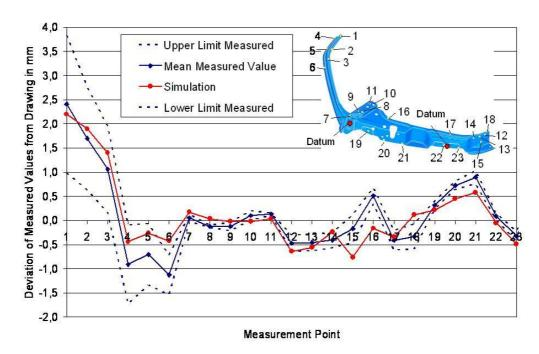
Figure 6: Comparison of the measured and calculated deviation from the required design geometry for 23 measuring points of the rear body lock panel.
