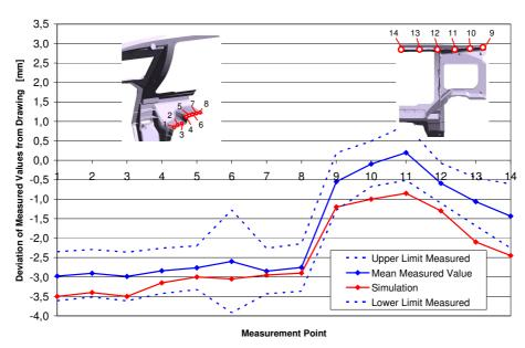
Figure 11: Comparison of the calculated and measured distortions of the bulk head after heat treatment.
