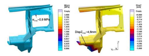
Figure 10: Stresses and deformation of the bulk head after solution heat treatment. The original geometry of the bulk head is shown in semi transparent grey.
