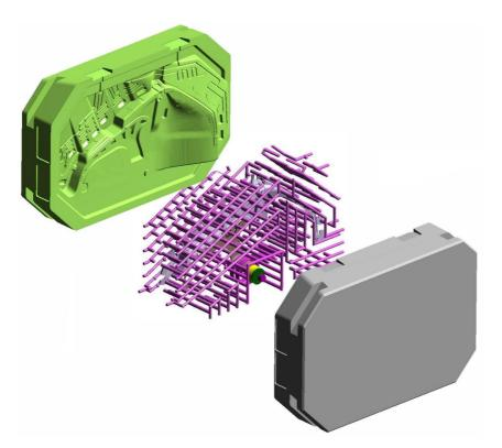
Figure 2: Geometry of the component including runner system, water cooling and oil tempering control channels, and the two die halves
