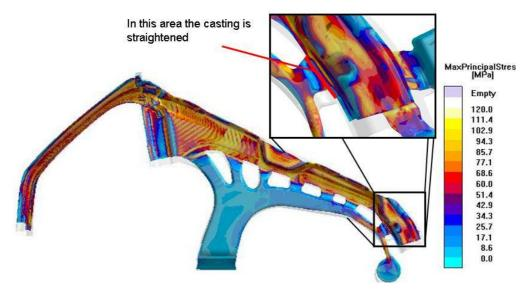
Figure 3: Maximum Principle Stress in the rear door lock panel casting just before ejection. The original geometry is shown as semi transparent grey, as well as the deformed geometry showing the relative shape change and areas of contact and constraint.
