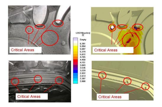
Figure 13: Comparison of the calculated die life (right) with the actual crack pattern in the area of the gate and the swan neck (left). The most critical areas are marked with red circles.
