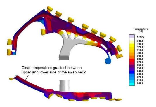
Figure 4: Temperature distribution in the casting and runner at ejection.
