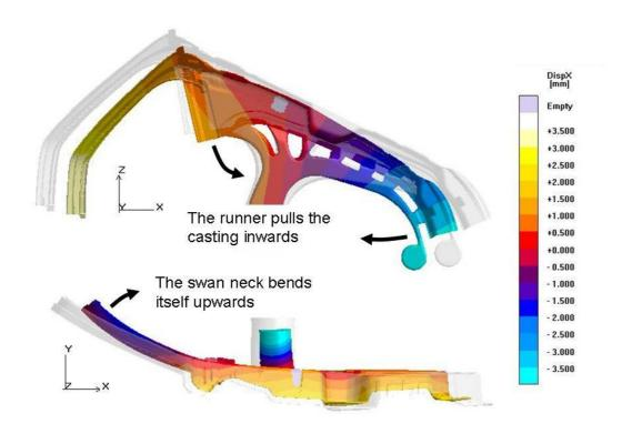
Figure 5: Deformation of the casting after cooling to room temperature shown as displacement from the starting point in the x direction. The original geometry is shows as semi transparent grey with the deformed geometry coloured.
