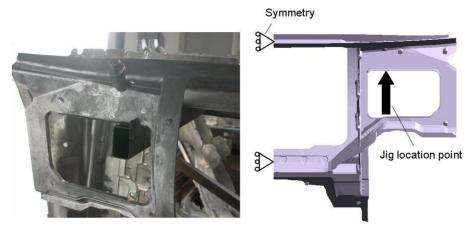
Figure 9: Jig location points the bulk head during heat treatment.
