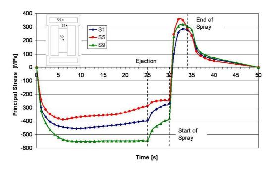
Figure 12: Typical stress changes for three points in the die surface during one casting cycle.
