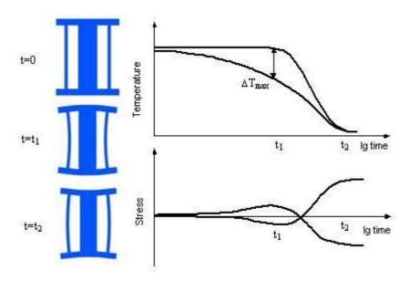
Figure 1: Formation of residual stresses and distortion in a stress lattice
