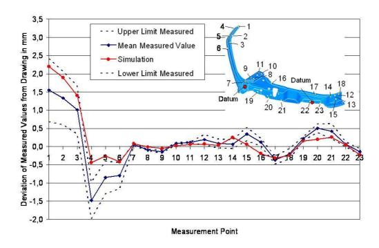
Figure 7: Comparison of calculated and measured distortion after clipping.
