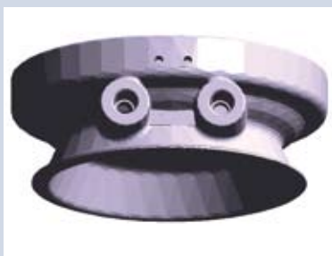
Front view of the flange. The bolt-on pieces are critical to shrinkage porosity.
