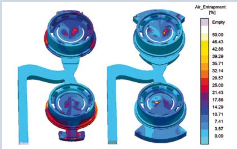
Air distribution in the casting after filling before (left) and after (right) optimization
