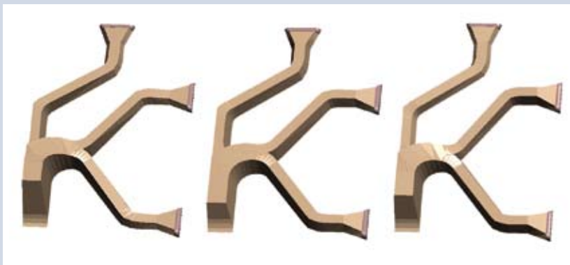
Three different variants of a running system. The parametric geometry supports variations of the cross sections of runner and gates at any required position.
