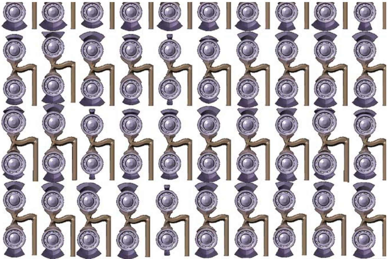
Today, hundreds of different gating systems and overflow wells can be assessed overnight by automatic optimization. The computer lists all variants, simulates the casting process and automatically finds the optimum variant. (Photo: MAGMA)
