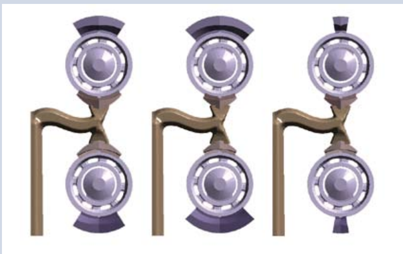
Three different variants of the geometry of gates and overflow tabs. The angle around the casting and the extension of the overflow tabs are varied.
