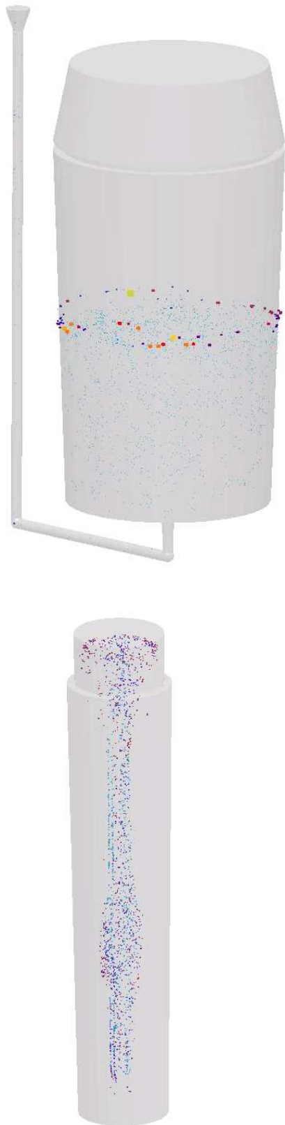
Fig. 5: Reoxidation particles are formed during teeming by contact of the steel melt to air. After their formation they move with the melt flow. Additional air contact allows them to grow and in addition agglomeration mechanisms take place. It is desired that the particles of a critical size float to the top surface of the melt. The upper picture shows
