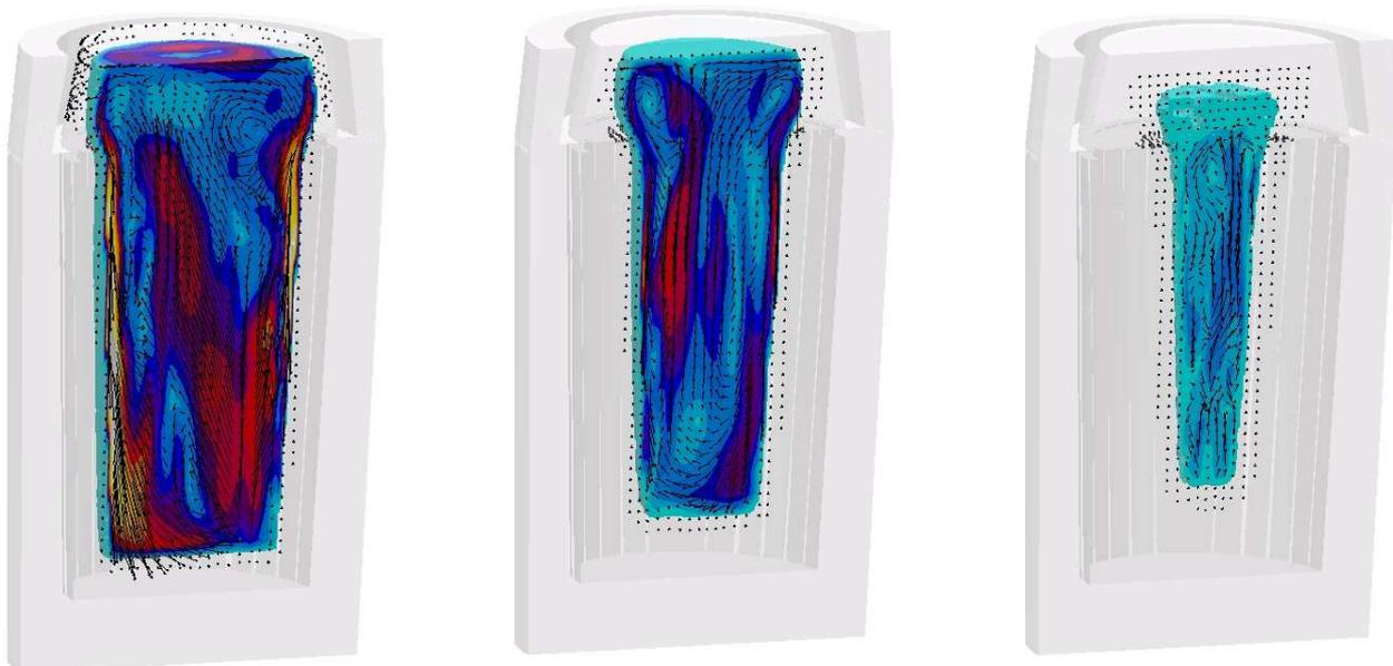
Fig. 3: With advancing solidification, thermo-solutal convection occurs in a progressively smaller area and thus is dampened by the solidifying structure. The left picture shows the convective flow velocities for the 40% solidified ingot, the middle picture shows the velocities for 65% and the right picture for 85% of solidification. Vectors illustrate the local flow directions.
