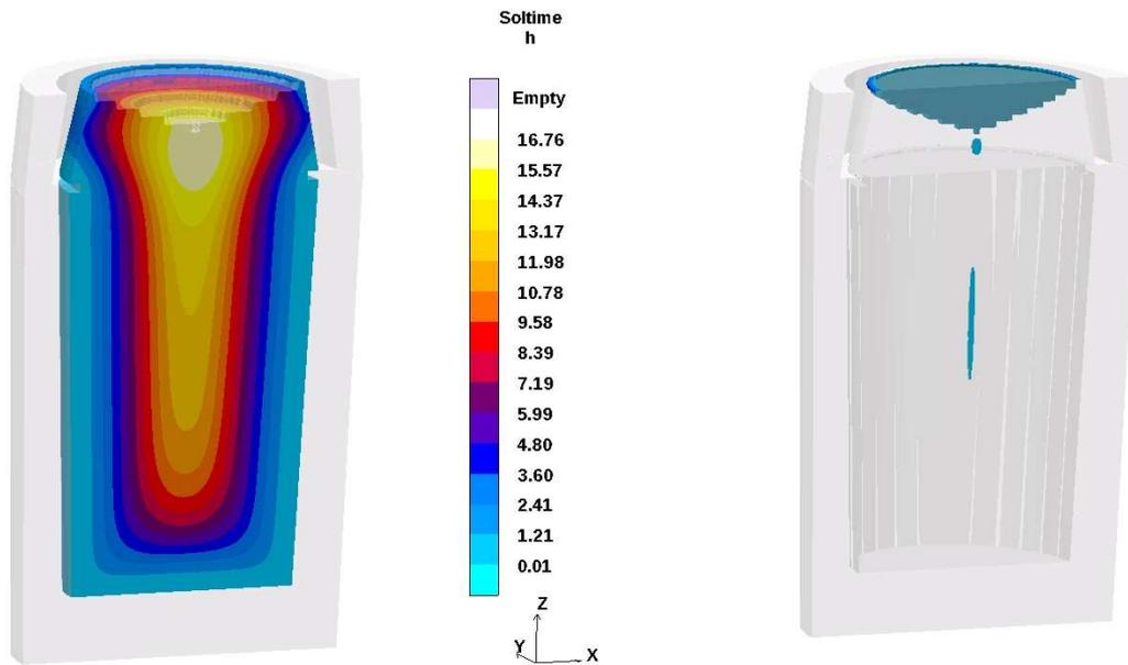
Fig. 2: Simulation allows monitoring of the solidification process in detail – the left picture shows the local solidification times for the ingot in a sliced view. The right picture shows the shrinkage cavity and the porosity that result for the given ingot under the assumed conditions
