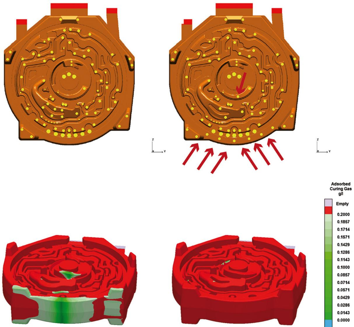
**Figure 12:** Comparison of gassing efficiency between the original (a) and the improved venting configuration (b). The manipulation of the gas flow leads to the sufficient flooding of the entire core.
