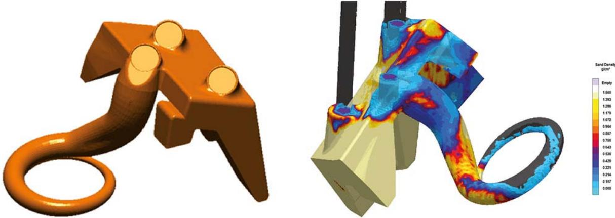
**Figure 1:** Turbocharger core geometry (a) and sand/binder mixture density distribution during the core shooting process (b).
