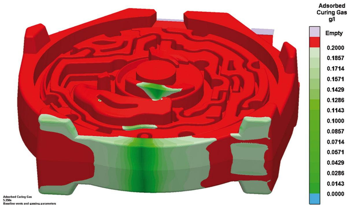
**Figure 11:** Amine gassing simulation. The concentration of absorbed amine is shown indicating the degree of curing. Completely cured areas are shown in red, incompletely cured areas in green (the darker the green, the less cured).
