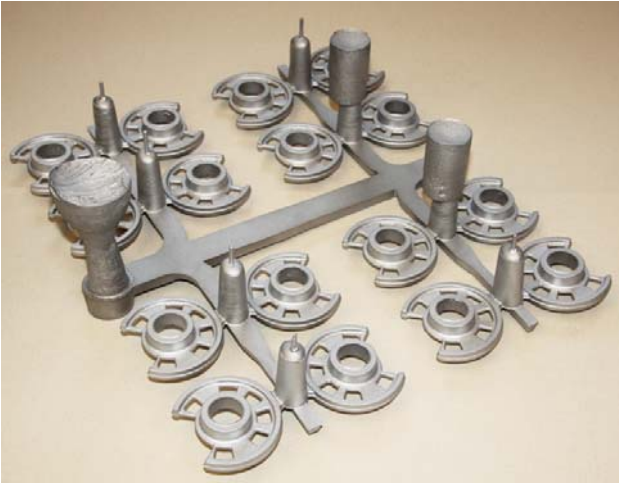
Fig. 11. Real casting after the autonomous optimization project was implemented. All casting defects experienced - mainly due to oxides - were eliminated in this project.
