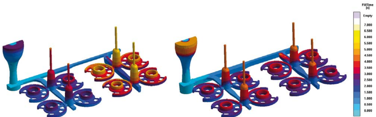
Fig. 5. Comparison of the filling time results between a "bad" (left) and a "good" (right) runner design. Filling times in the left design are significantly different than the filling times on the right - almost optimal - design.
