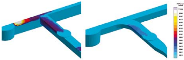
Fig. 6. Comparison of flow conditions between various gating designs. Criterion used is air pressure in [mbar] unit. All light colored areas show various levels of air entrapment inside the gating systems.
