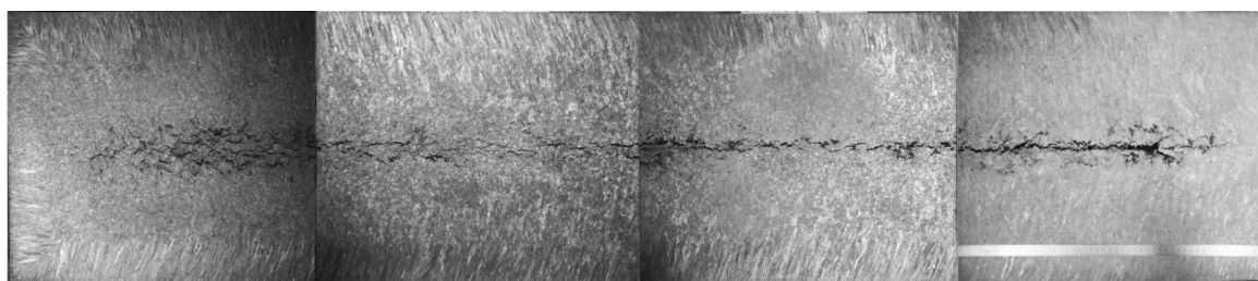
Fig. 3 Results from casting trial showing presence of porous areas and microstructure of the ingot (Courtesy of Trinecke zelezarny, a.s.). The bottom of the ingot is on the left hand side of the image.
