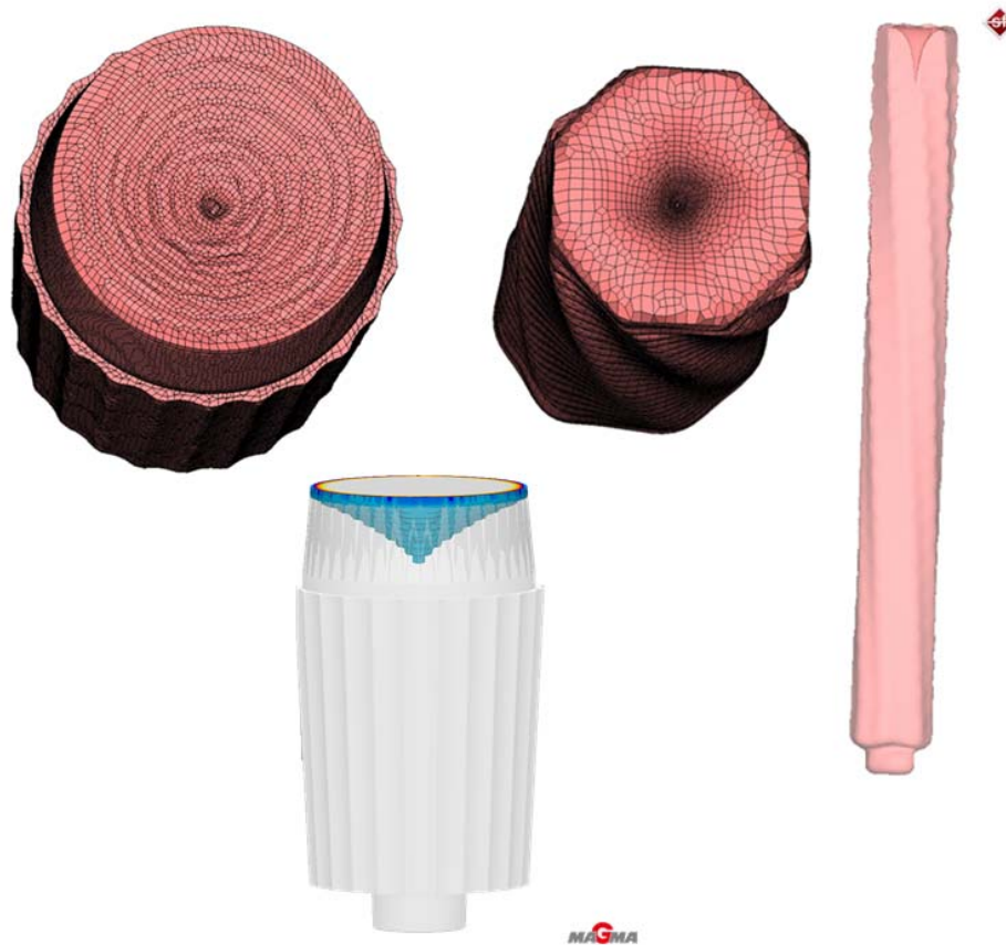
Fig. 3: Shrinkage cavity at the beginning of the cogging process (as predicted by the casting process simulation) (left) and at the end (right)
