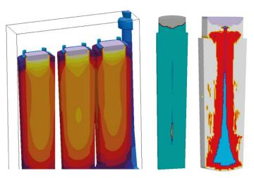
Ingot and mold temperatures in the cluster (left); porosity indications, CET zone (right)
