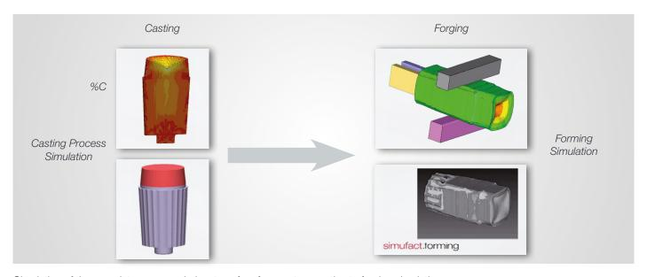
Simulation of the complete process chain - transfer of as-cast properties to forging simulation
