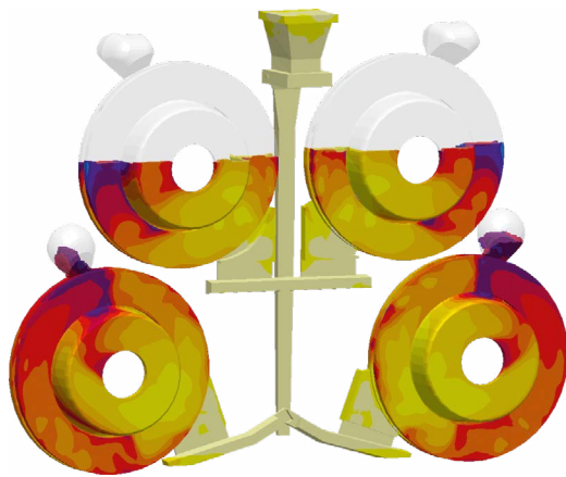
Mold filling of four gray iron brake discs
