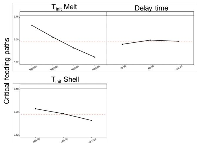
Main Effects Diagram: Influence of process parameters on the feeding behavior in the component
