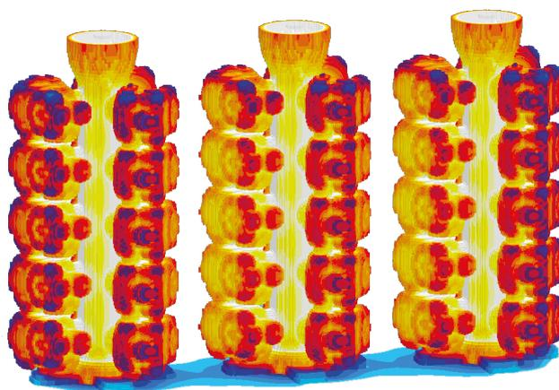
*Radiation between heated shell molds and with the environment*
