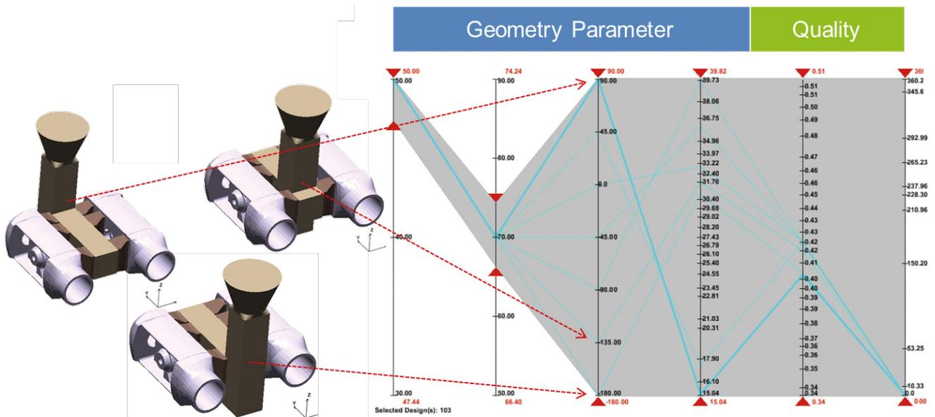
Parallel Coordinates Diagram: Evaluation of different geometries on the selected quality criterion (porosity) in a Design of Experiments
