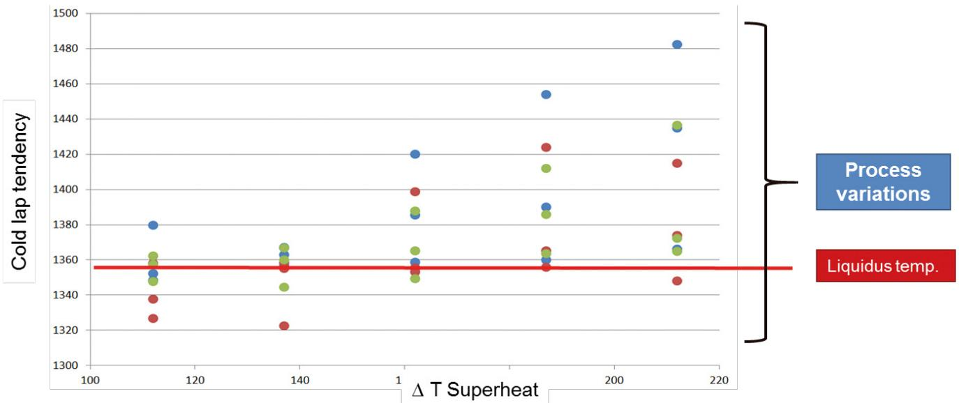
Determination of the risk for cold shuts as a function of process variables and fluctuations
