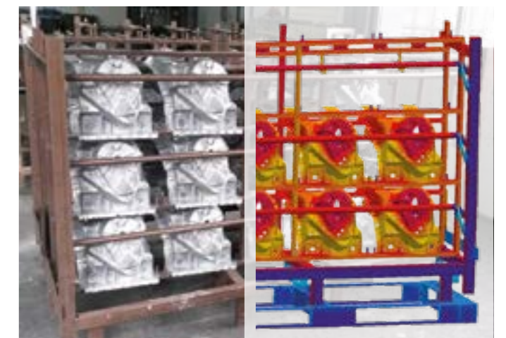
Simulation of cast parts positioned in a heat treatment rack as in the real process
