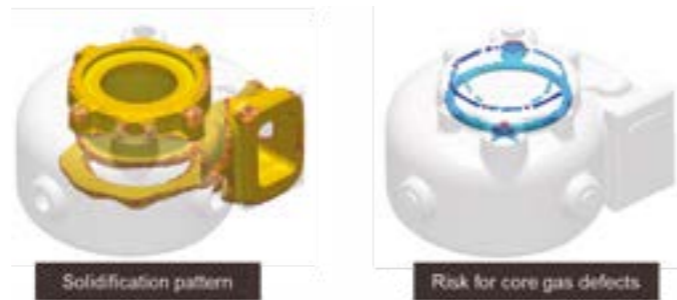
Risk areas for core gas defects depending on local solidification conditions and binder decomposition
