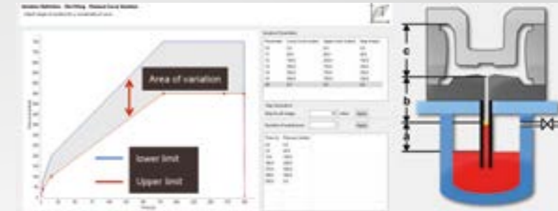
Assistants for fast and easy estimation of pressure conditions for filling the stalk, casting and cavity
