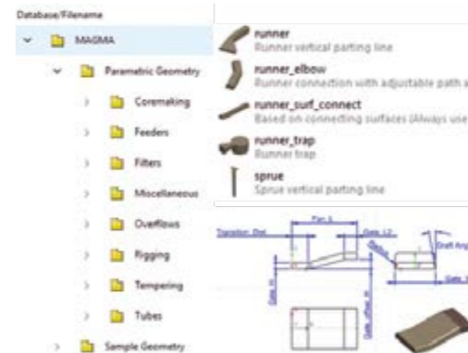
Comprehensive database with fully parametric geometries for all essential elements of the gravity die casting process
